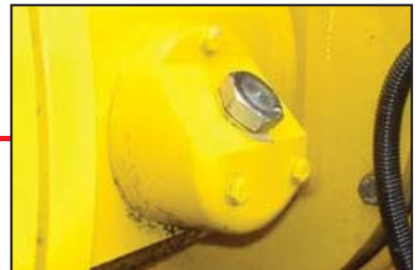
Failsafe oil filling - impossible to overfill. Either side filling option.
